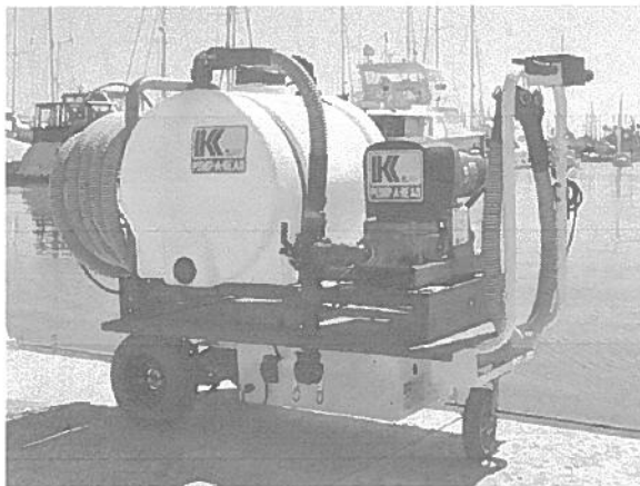
Figure 1 Example mobile sewage pump-out cart on a floating marina
