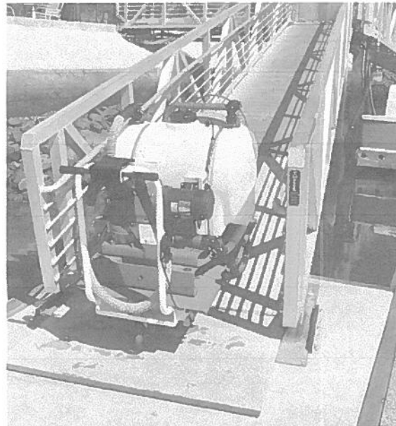
Figure 2 Mobile sewage pump-out cart on a hinged gangway leading from a floating marina to land
